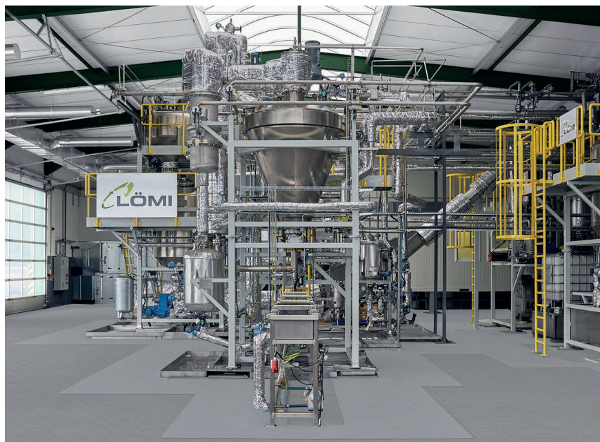
Fig. 2. The demonstration plant of Lömi GmbH processes up to 25 kg of different waste fractions per hour. © Lömi
